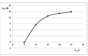
Fig.2. Voltage Gain with Negative Feedback versus Supply Voltage for UBCT Cascode Amplifier
