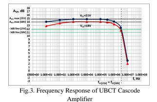
[Circuit specifications: UBCT [JFET BFW10, BJT CL100 and ( $R_S$ - $R_E$ ) resistor pair (100 $\Omega$ -10 $\Omega$ )], BJT CL100, ( $R_1$ - $R_2$ ) resistor pair (4.7 $k\Omega$ -10 $k\Omega$ ),  $R_G$ =1M $\Omega$ ,  $R_L$ =1 $k\Omega$ ,  $R_{SF}$ =100 $\Omega$ ,  $C_{IC}$ = $C_{OC}$ =10 $\mu$ F,  $C_{BB}$ =10 $\mu$ F,  $C_{SB}$ =N/C,  $V_I$ =100m $V_{P-P}$ , f=10Hz-10MHz, T=31°C-33°C].
