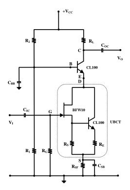
Fig.1. Circuit Design of UBCT Cascode Amplifier
